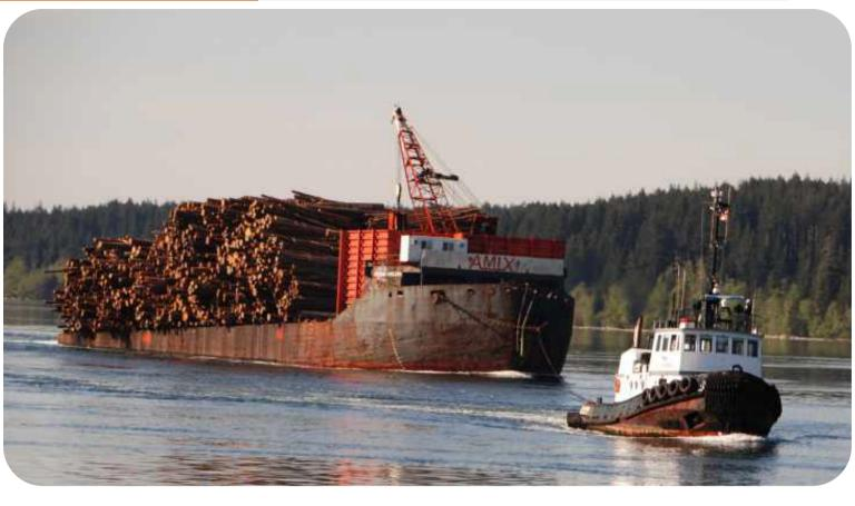
The **Ocean Oregon** is a cargo barge with a wood deck. The barge is used for log barging and project cargo.
